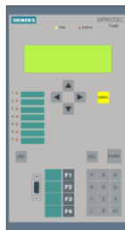
Figura 6.9 – Relé SIPROTEC 7SJ62
