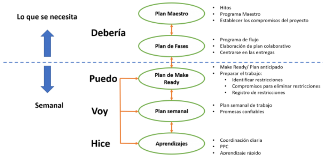
Figura N° 7: Diagrama Last Planner System
