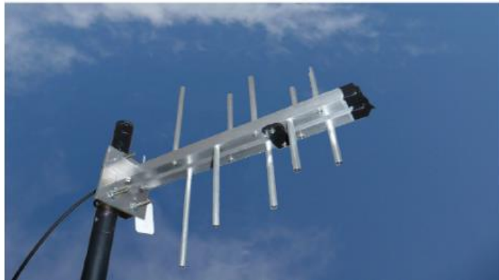
Figura 29: Log Periodic Directional UHF Antenna for Rural Connect® CPE
