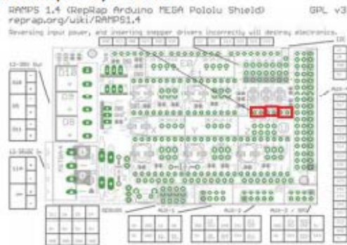
From left to right: Extruder 1 thermistor, heat bed thermistor, and extruder 2 thermistor
