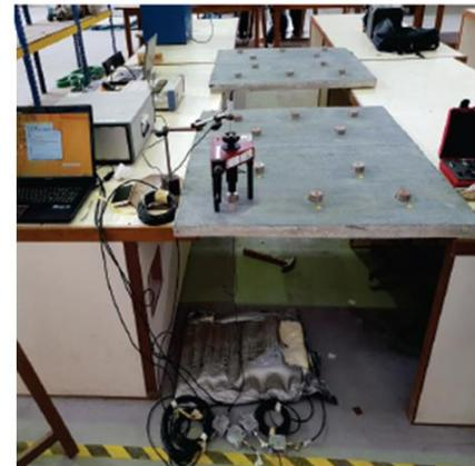
Fuente: “Acoustic emission signals of pull-off test for concrete slab strengthened with CFRP using various surface preparations”, Md et al, (2019)
