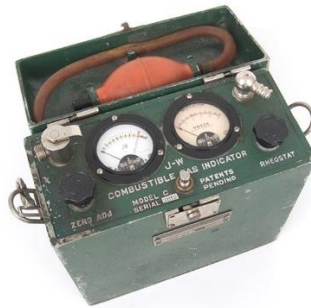
Figura 8. Monitor de LEL Model C (1929) Fuente: RKI Instruments (2006). Gas detection history
