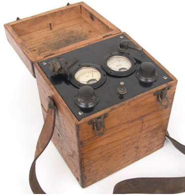
Figura 7. Monitor de LEL Model B (1927) Fuente: RKI Instruments (2006). Gas detection history
