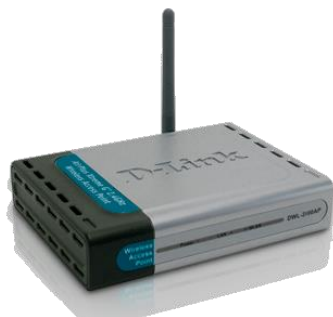
FIGURA 2.19. Access Point Link
