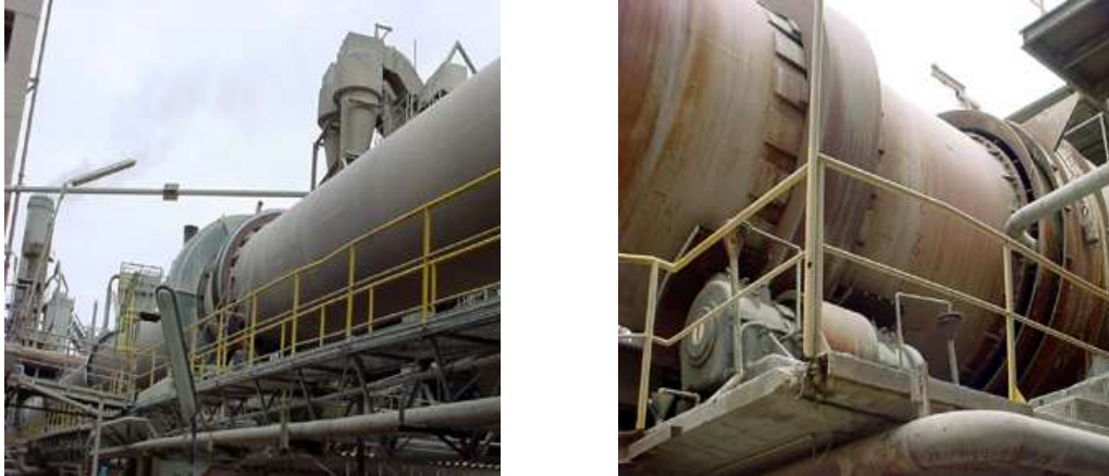
Figura 4: Horno rotativo 2 - (03.m01991), diam. 3.60 m x 50.0 m
