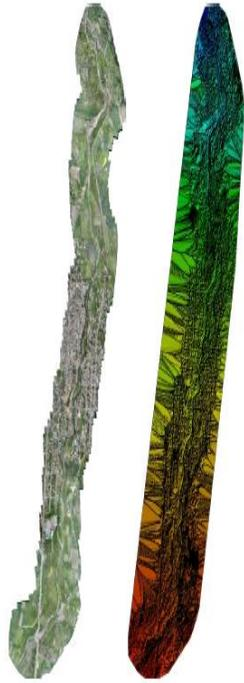
Figure 1: Orthomosaic and the corresponding sparse Digital Surface Model (DSM) before densification.
