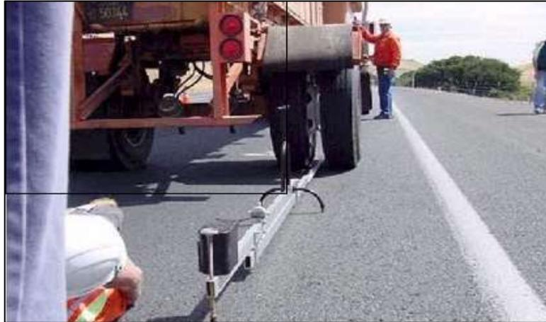
Figura N°29: Viga Benkelman
