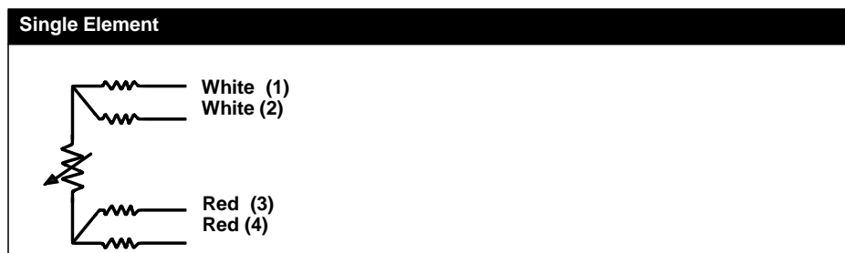
Figure 3-5. Rosemount 68Q, 78 Standard Temperature Range, and 58C RTD Sensor Lead Wire Configurations
