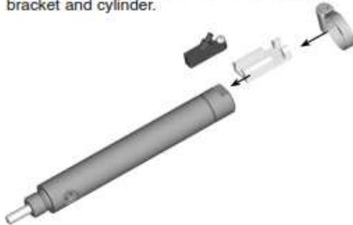
2. Tighten band clamp, loosen Phillips head screw, insert switch into bracket, and then tighten.
