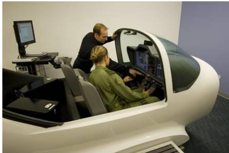
Figura 17. Cockpit procedure trainer
