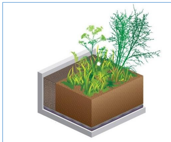
Figura 13: Techo semi-intensivo Fuente: Sud Sostenible, 2013, ( http://i1.wp.com/sudsostenible.com/wp-content/uploads/2013/12/semi-intensiva.jpg?w=545 )
